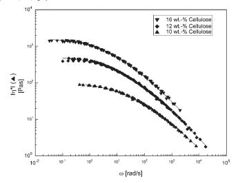
**Figure 1.** Rheology master curves of 10, 12 and 16 wt.-% cellulose (Linters, DP 795) dissolved in EMIM acetate (reference temperature 95 °C).
